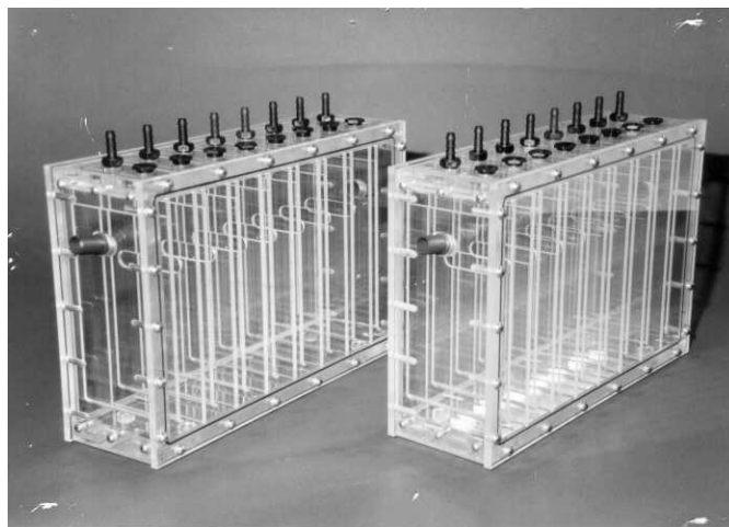
Figure 3.1: 10 ℓ Perspex laboratory-scale ABRs showing inlet, internal baffles, gas vents and sampling ports
