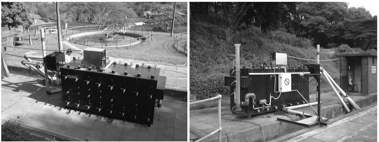
Figure 3.7: Photographs of the front and back of the pilot ABR installed at Umbilo WWTP
