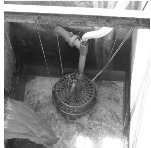
Figure 3.8 Installation of the ABR at Kingsburgh WWTP. The outlet end of the pilot ABR showing the membrane unit attached to the last compartment (left); and a laundry basket housing the submersible pump in a wastewater sump near the feed end of the ABR (right)
