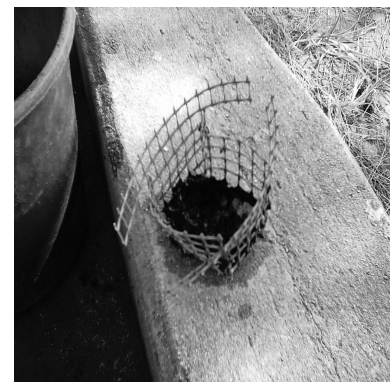
Figure 3.9: Modified outlet of the ABR showing mesh for preventing coarse solids entering the flow meter.
