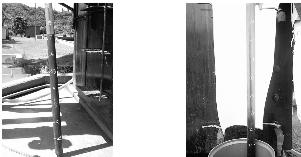
Figure A1. 1: Core Sampler filled with compartment 1 sludge (left) and compartment 8 sludge and supernatant (right)
