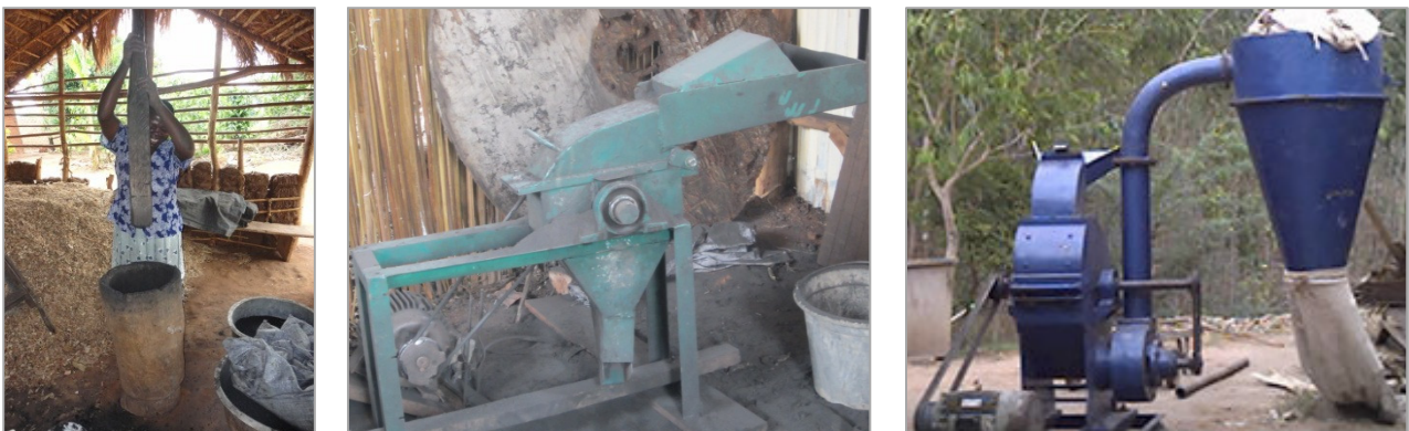
Figure 4: From left-right: Ugandan micro-entrepreneur manually grinding large charcoal fines into dust for briquetting; Locally fabricated electric grinding machine costing approximately US$2,000 in Uganda; Industrial Hammer Mill Grinder similar to those used by larger-scale briquetting companies in East Africa such as Chardust Ltd. This type from SREE Engineering Works, India, has capacities of 200 – 1,500 kg/hr at a cost of US$3,000-13,300.
