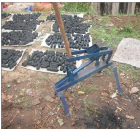
Figure 9: From left-right: Manual Extruder, Alfatar Industries, Nyeri, Kenya; Manual Screw Extruder, Uganda; D-Lab hand briquette press(image source: Engineering for Change )
