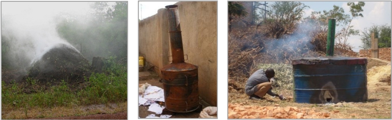
Figure 3: From left-right: traditional open air carbonisation method; top-lit-down-draft (TLUD) steel kiln; ARTI steel drum retort ( www.arti-africa.org )
