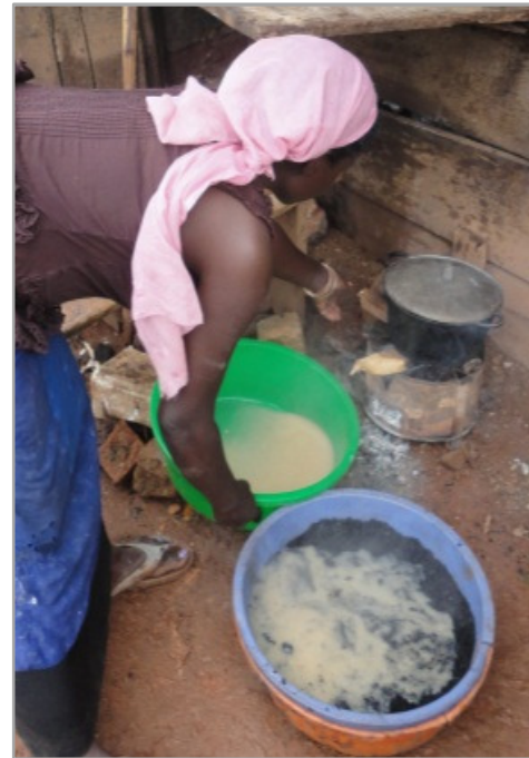
Figure 5: Mixing cassava flour as a binder for charcoal dust
