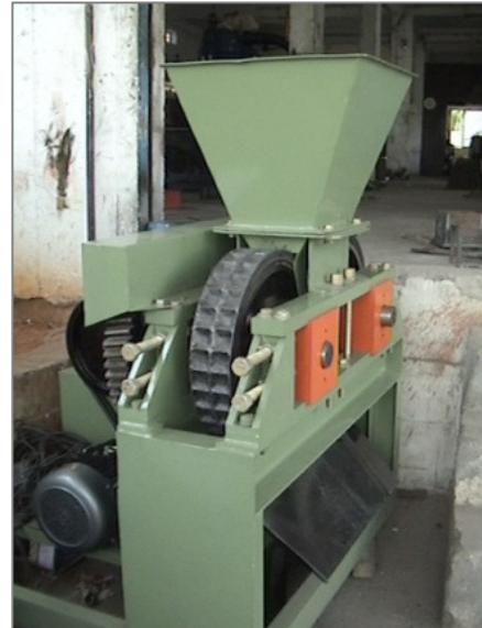
Figure 8: Roller Press, SREE Engineering Works, India
