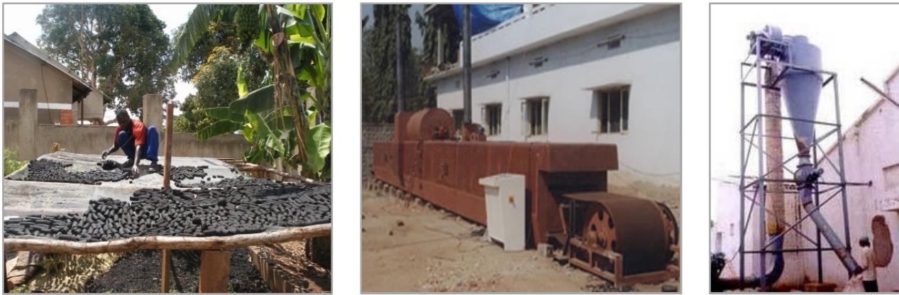
Figure 6: From left-right: briquettes sun drying on raised wire mesh in Uganda; Tunnel Drier for briquettes and a Flash Drier for feedstock (both SREE Engineering Works in India)
