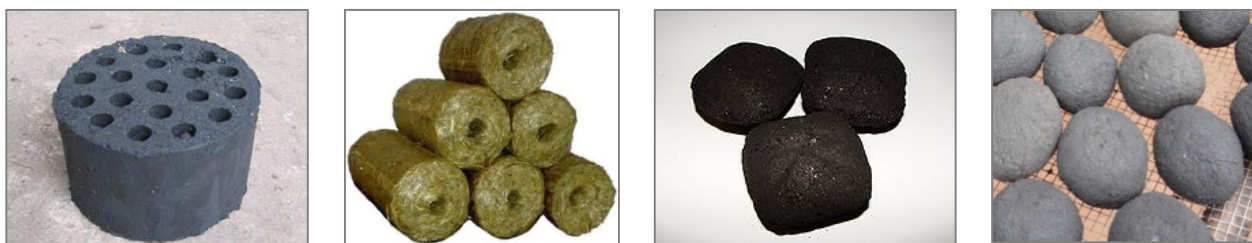
Figure 2: From left-right: honey-comb briquette (hydraulic press); non-carbonised straw briquette (piston-extruded); carbonised charcoal dust (roller press); hand-made charcoal dust briquettes
