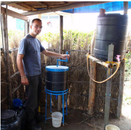
Struvite from urine researched in field laboratory setting (Photo: EAWAG).
