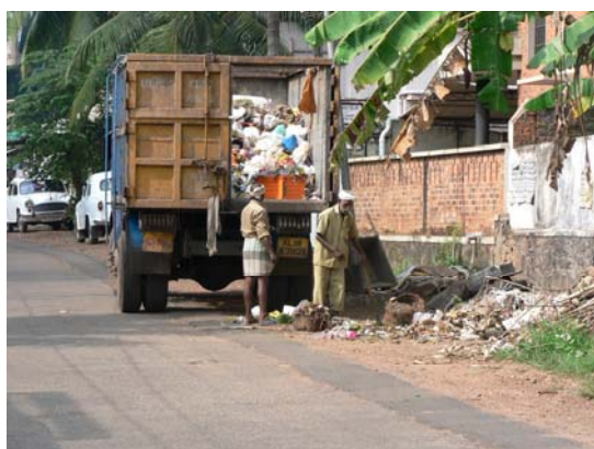
Figure 2: Collection of waste at an open waste collection point. The waste is dumped on the ground at special places along the roads and then collected by municipal or private workers (Picture: Florian Heeb).
