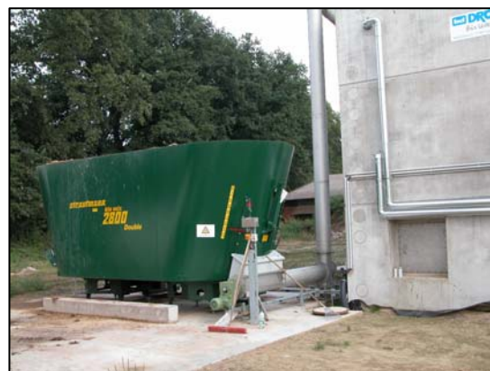
Figure 3. Feeding Corn Silage to the Digester
